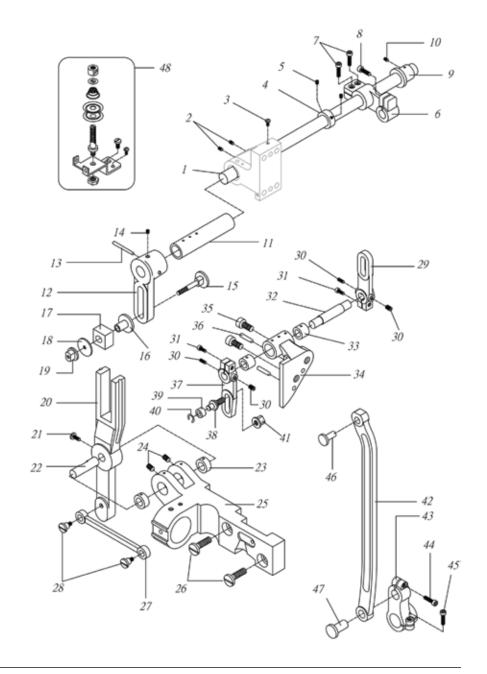
Upper Feed Mechanism Components 8
